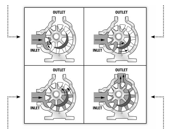
As the rotor continues to turn, the liquid is forced past the crescent shaped area and moves towards the discharge port. As the rotor completes one complete rotation, the rotor and idler teeth interlock forcing the liquid through the discharge of the pump. The pump may take several rotations to completely prime depending on the conditions of the application.
